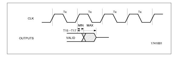
Figure 2–4. Output Float Delay Timing
