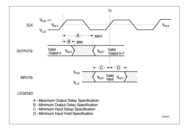
Figure 2–1. Drive Level and Measurement Points for Switching Characteristics
