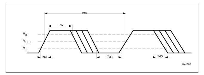
Figure 2-6. TCK Timing and Measurement Points
