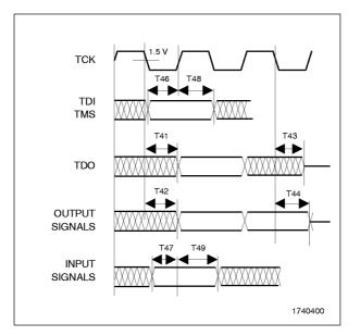
Figure 2–7. JTAG Test Timings
