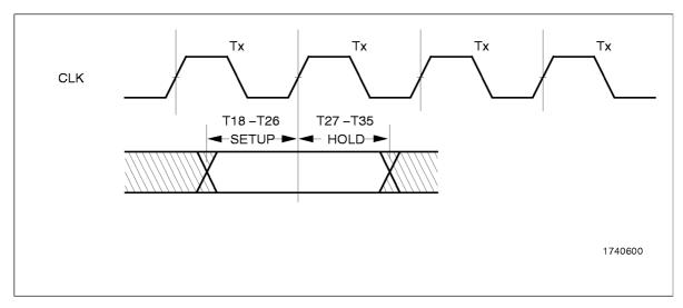
Figure 2–5. Input Setup and Hold Timing
