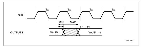
Figure 2–3. Output Valid Delay Timing
