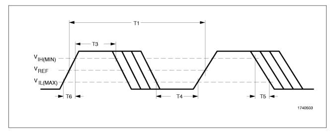
Figure 2–2. CLK Timing and Measurement Points
