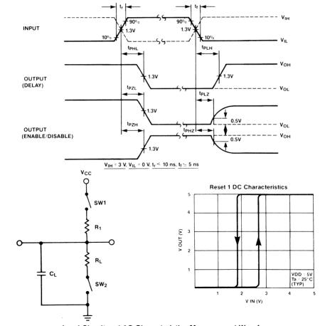
Load Circuit and AC Characteristics Measurement Waveform
