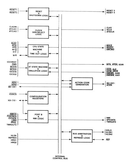
Figure 1-1. 82C301 Functional Block Diagram
