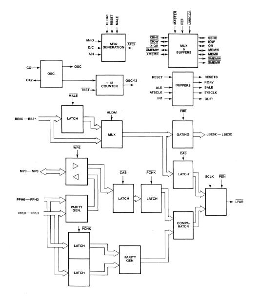
Figure 6-1. 82A306 Functional Block Diagram
