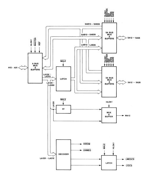
Figure 3-1. 82A303 Functional Block Diagram
