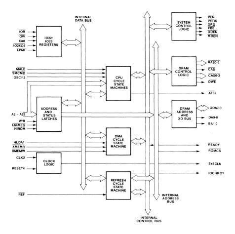
Figure 2-1. 82C302 Functional Block Diagram
