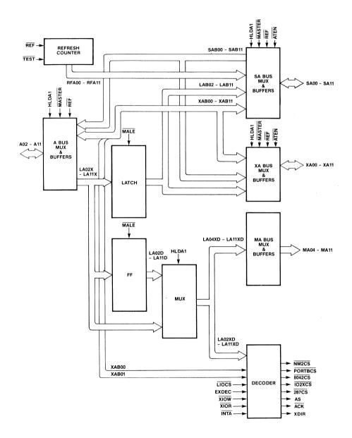
Figure 4-1. 82A304 Functional Block Diagram
