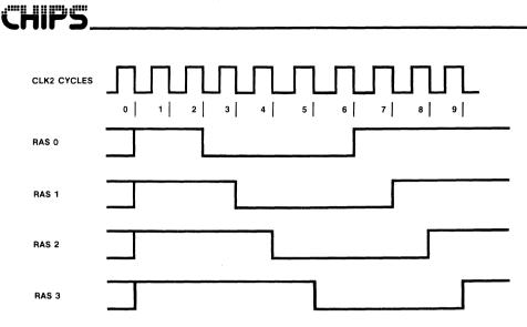
Figure 2-3. Staggered RAS pulses during refresh
