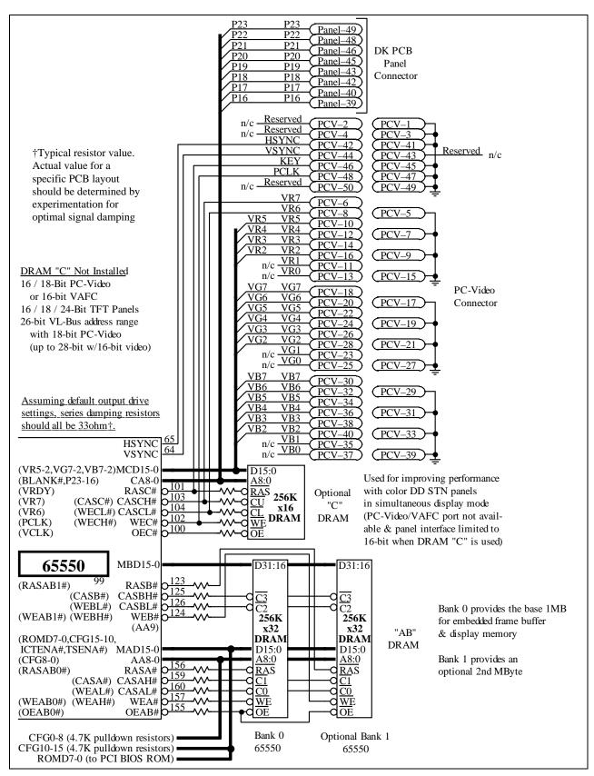
Figure 16-7: Circuit Example 256Kx32 Display Memory Interface
