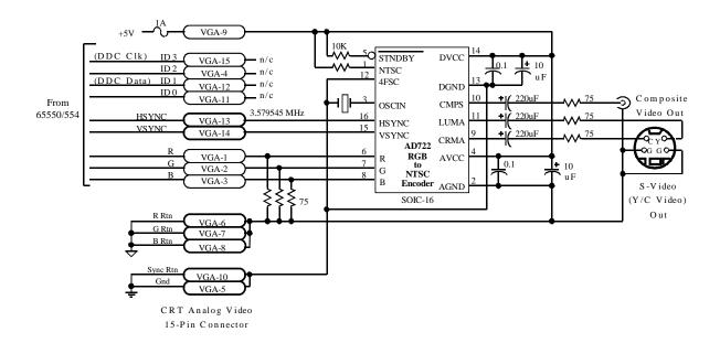
Figure 16-10: Circuit Example RGB-to-NTSC Encoder
