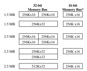
Figure 1-2: Display Memory Configurations with an STN-DD Buffer
