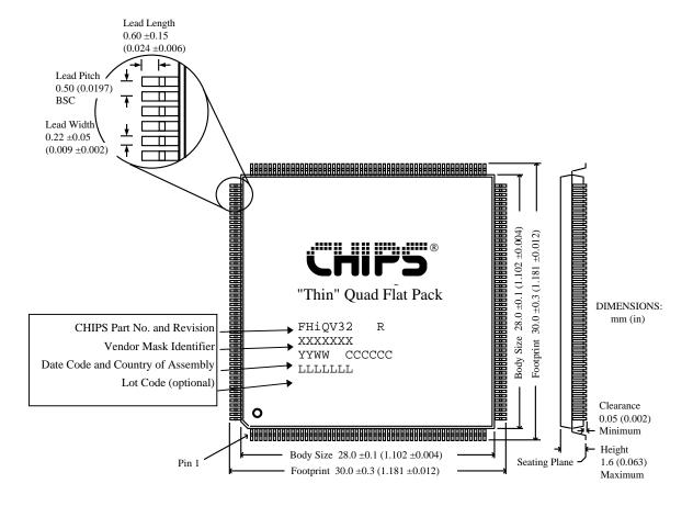
Figure 18-1: Thin Quad Flat Pack (TQFP)
