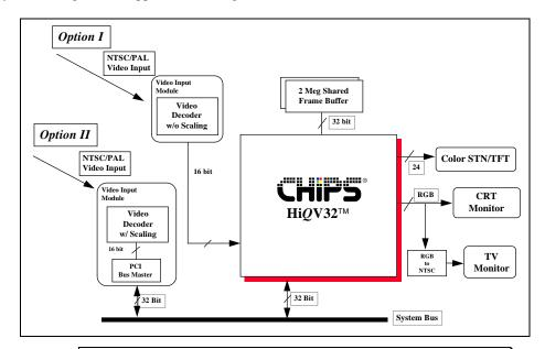
Figure 1: System Diagram - External Interfaces
