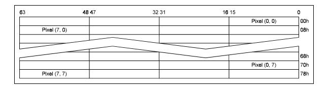
Figure E-3-6: 16bpp Pattern Data -- Occupies 128 Bytes (16 Quadwords)
