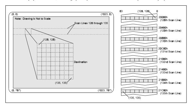
Figure E-4-4: On-Screen Destination for Example Character Drawing BitBLT
