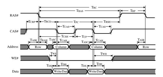
Figure 17-9: DRAM Page Mode Write Cycle Timing
