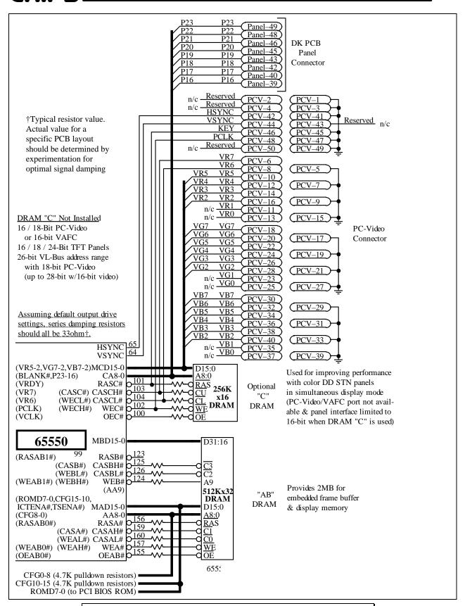
Figure 16-8: Circuit Example 512Kx32 Display Memory Interface
