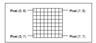
Figure E-3-3: Pattern Data -- Always an 8x8 Array of Pixels
