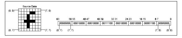
Figure E-4-5: Source Data in System Memory for Example Character Drawing BitBLT
