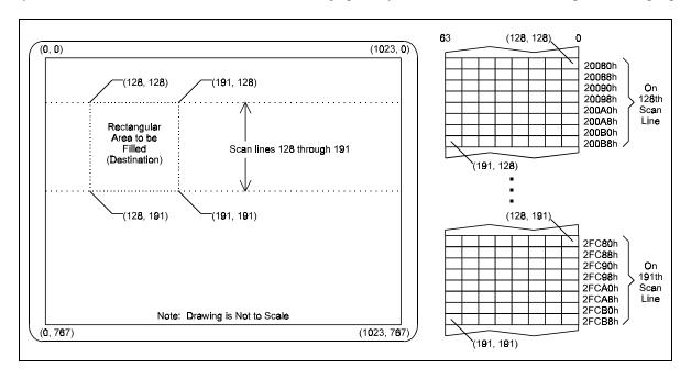
Figure E-4-1: On-Screen Destination for Example Pattern Fill BitBLT
