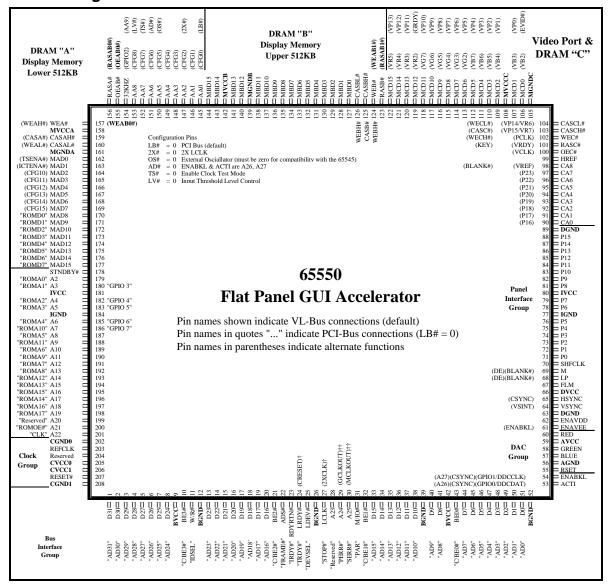
Figure 2-1: Pin Diagram
