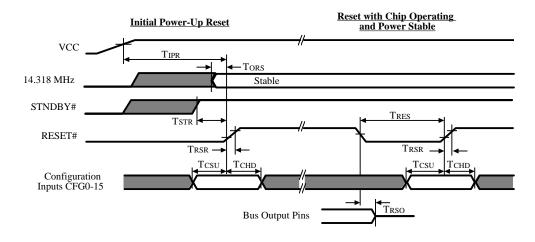
Figure 17-4: Reset Timing
