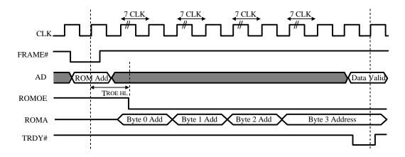
Figure 17-7: PCI BIOS ROM Timing
