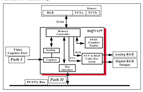
Figure 2: Internal Data Flow
