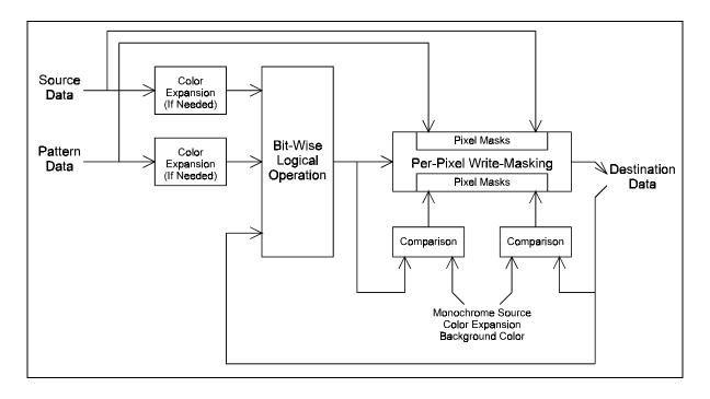
Figure E-1: Block Diagram and Data Paths of the BitBLT Engine
