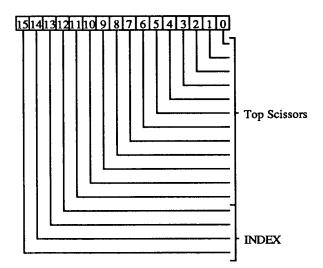
11-0 Top Scissors is the minimum Y coordinate value for the scissors rectangle.
