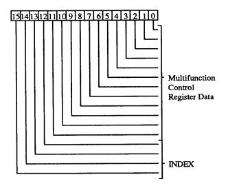
11-0 Multifunction Control Register Data. The MULTIFUNC\_CNTL register is the index to a set of registers at the same address. The INDEX bits are used to determine which of the nine currently implemented registers is being written to. This data field is defined for each of the indexed registers in the pages to follow.
