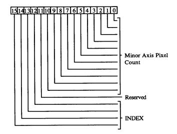
Minor Axis Pixel Count is used to define the height for BITBLT and rectangle commands. The actual height is:
