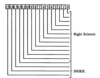
11–0 Right Scissors is the maximum X coordinate value for the scissors rectangle.
