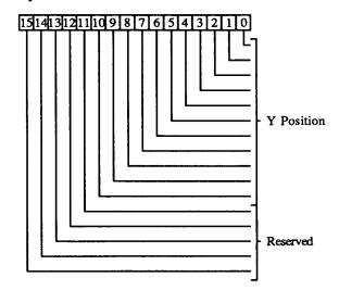
11-0 Y Position = Y coordinate of current position (in pixels). The XY position is relative to the top left corner of the display. Each scan line displays X-coordinates 0 through XMAX - 1. Each screen displays Y-coordinates 0 through YMAX - 1.
