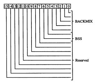
4-0 BACKMIX The background mix defines the mix or raster op to be used in drawing operations. It is analogous to the Foreground Color Mix. One of these two mixes is selected for each pixel in the current nugget based on the PIX\_CNTL register. All 16 logical mixes, and five arithmetic mixes (sum, difference, min, max, and average) are supported. Options also exist for sum, average, and difference mixes to
