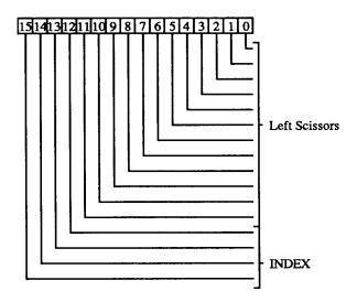
**11–0** Left Scissors is the minimum X coordinate value for the scissors rectangle.
