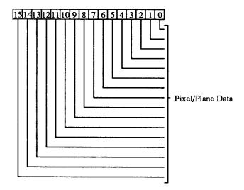
15-0 Pixel/Plane Data In through planes mode (PLANAR=0), bits D7:0 and D15:8 map onto bit planes 7:0 of an individual pixel. In across planes mode (PLANAR=1), bits D4:0 and D12:8 map onto pixels 0:4 within a nugget (1 bit per pixel).
