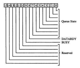
7-0 Queue State indicates the number of positions available in the queue. The standard 8514/A command queue is eight bytes deep. Queue State is nicknamed the thermometer register. It shows the number of bytes available encoded linearly. Queue State = 0 if the queue is empty; this does not imply that the 82C480 is idle-it may have consumed all of the data in the command queue but still may be executing a drawing command. Always test BUSY to determine if the drawing engine is idle.
