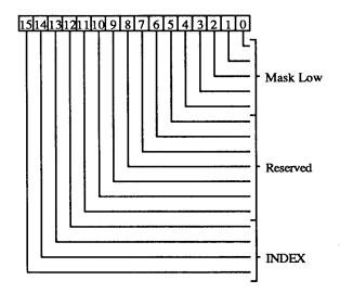
4-0 Mask Low is used to select the mix on a pixel by pixel basis. If MIXSEL = 01, then the pattern registers are used to select foreground or background mix. Mask Low applies to even numbered nuggets (0 is leftmost on the screen); Mask High is applied to odd numbered nuggets.
