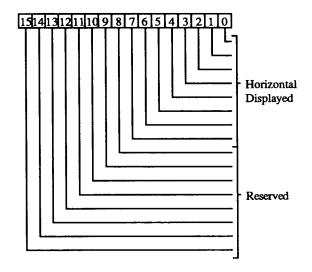
7-0 Horizontal Displayed defines both the number of displayed pixels per scan line and the start of the horizontal blanking. All horizontal timings are performed in terms of double nuggets. The start of the horizontal blanking signal occurs at:
