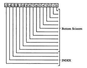
11-0 Bottom Scissors is the maximum Y coordinate value for the scissors rectangle.
