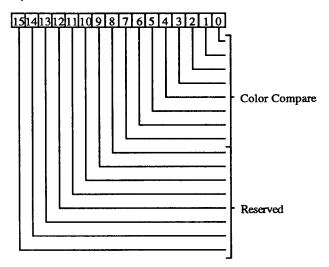
7-0 Color Compare defines an 8-bit color which is compared to the destination data during BitBlts. The arithmetic comparison to be used (<,>,=,true,false, etc..) is specified by the COLCMPOP bits of the PIX\_CNTL register (MFC[A][5:3]).
