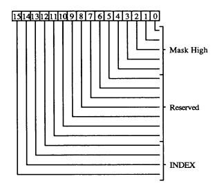
4-0 Mask High is used to select the mix on a pixel by pixel basis. If MIXSEL=01, then the pattern registers are used to select foreground or background mix. Mask High applies to odd numbered nuggets (0 is leftmost on the screen); Mask Low is applied to even numbered nuggets.
