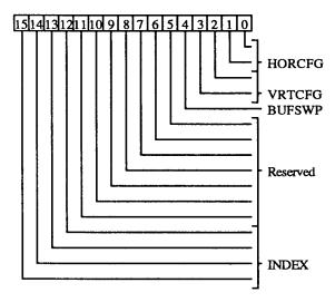
1-0 HORCFG This field contains information which the 8514/A uses to determine the X-Coordinate divisor. Bit 0 is used to indicate 5-pixel operation and should only be set if EC2[11] = 1 (the 5PN bit). Bit 1 determines if the VRAMs are interleaved in the horizontal direction. The interleave table results in the following:
