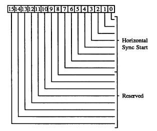
7-0 Horizontal Sync Start defines the timing delay of the horizontal sync signal from the start of a scan line. For HSYNC to occur, H\_SYNC\_STRT must be less than H\_TOTAL. The horizontal sync pulse begins at:
