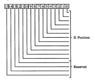
11-0 X Position = X coordinate of current position (in pixels). The XY position is relative to the top left corner of the display. Each scan line displays X-coordinates 0 through XMAX - 1. Each screen displays Y-coordinates 0 through YMAX - 1.
