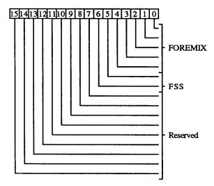
4-0 FOREMIX The foreground mix defines the mix or raster op to be used in drawing operations. It is analogous to the Background Color Mix. One of these two mixes is selected for each pixel in the current nugget based on the PIX\_CNTL register. All 16 logical mixes, and five arithmetic mixes (sum, difference, min, max, and average) are supported. Options also exist for sum, average, and difference mixes to
