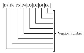
This register contains the version number for the 82C450. Values start at 40h and are 7-0 incremented for every silicon step.
