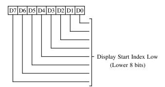
**7-0** Lower 8 bits of the display start address. The display start address points to the memory address corresponding to the top left corner of the screen.
