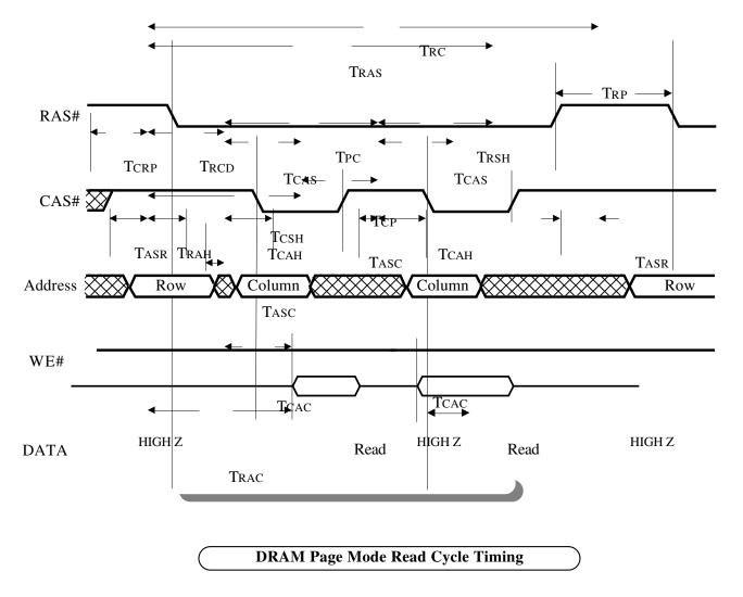
Note: The above diagram represents a typical page mode read cycle. The number of actual CAS cycles may vary. The maximum number of CAS cycles allowed is 32 (when the FIFO is being filled).
