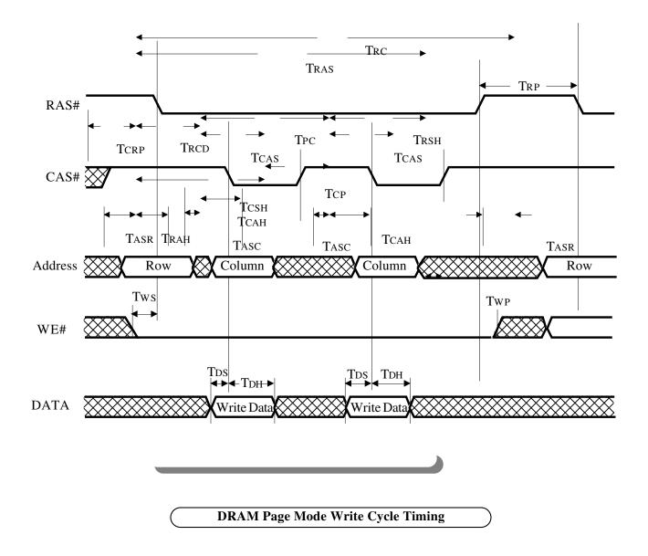
Note: The above diagram represents a typical page mode write cycle. The number of actual CAS cycles may vary between 0 and 4.
