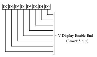
**7-0** These are the eight low order bits of a 10-bit register. The 9th and 10th bits are located in the CRT Controller Overflow register. The actual count = Contents of this register + 1.
