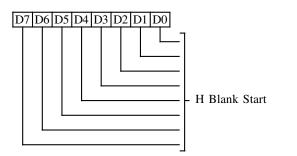
This register is used for all VGA and EGA modes. It is also used for 640 column CGA modes and MDA/Hercules text mode. In all 320 column CGA modes and Hercules graphics mode, the alternate register is used.
