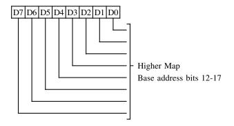
7-0 These eight bits define the Higher Map (in Dual Map Mode) base address bits 17-12. The map starts on a 1K boundary in planar modes and on a 4K boundary in packed pixel modes. This register maps the CPU window into display memory based on the contents of GR06 bits 2-3 as follows:
