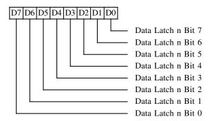
This register may be used to read the state of Graphics Controller Memory Data Latch 'n', where 'n' is controlled by the Graphics Controller Read Map Select Register (GR04 Bits 0 & 1) and is in the range 0-3.
