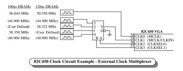
Note: any of the clock configurations shown on this or the following page are suitable for supporting digital monitors as well as analog monitors. The 82C450 has the capability to generate the required 14 and 16 MHz frequencies internally from the 50 and 28 / 56 MHz frequencies supplied by any of these circuits (see XR02 bit-1).
