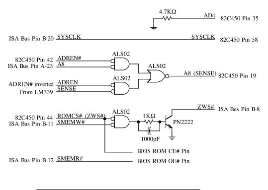
Block Diagram - ZWS Enhancement Circuit A
