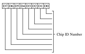
This register is only accessible in Setup Mode.
