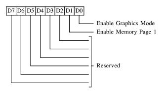
This register is effective only in Hercules mode. It is accessible in Hercules emulation mode or if the extension registers are enabled. It may be read back through XR14 bits 2 & 3. It is cleared by RESET.
