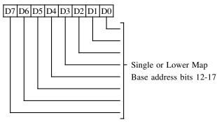
**7-0** These eight bits define the Single or Lower Map (in Dual Map Mode) base address bits 17-12. The map starts on a 1K boundary in planar modes and on a 4K boundary in packed pixel modes. In case of dual mapping this register controls the CPU window into the display memory based on the contents of GR06 bits 2-3 as follows:
