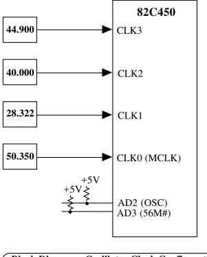
Block Diagram - Oscillator Clock Configuration 1
