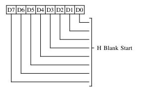
This register is used in low resolution (320-pixel) CGA modes and Hercules graphics modes.
