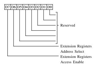
This register is only accessible in Setup Mode. It is cleared by RESET.
