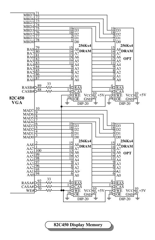
Note: For minimum configurations, two DRAMs may be implemented instead of four. In this case, the two optional DRAMs on the right side of the above circuit marked '**OPT**' may be removed.
