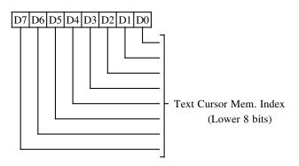
**7-0** Lower 8 bits of the memory address where the text cursor is active. In CGA/MDA/Hercules modes, this register wraps around at 16, 32, and 64 KByte boundaries respectively.
