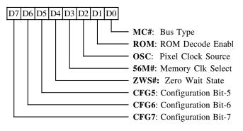
These bits latch the state of the CPU data bus (AD bus) on the falling edge of RESET. The state of bits 0-4 after RESET effect the 82C450 internal logic as indicated below; bits 5-7 are latched from AD5-7 on the falling edge of RESET and may be read in this register, but otherwise have no hardware effect on the 82C450 chip. The AD bus has internal on-chip high-valued pullups and will float high if not driven otherwise during RESET so that the default state of all bits is 'one'.
