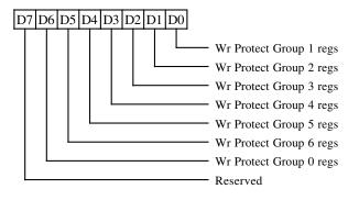
This register controls write protection for various groups of registers as shown. 0 = unprotected, 1 = protected.
