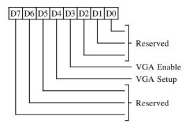
This register is used with the PC-Bus Interface only. It is cleared by RESET. In the Micro Channel interface, the Setup mode and VGA Disable are controlled through the SETUP# and DISA# pins, respectively.
