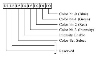
This register is effective only in CGA modes. It is accessible if CGA emulation mode is selected or the extension registers are enabled. This register may also be read or written as an Extension Register (XR7E). It is cleared by RESET.
