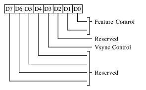
1-0 Feature Control. These bits are used internal to the 82C450 in conjunction with the Configuration Register (XR01). When enabled by XR01 bits 2-3 and Misc Output Register bits 3-2 = 10, these bits determine the pixel clock frequency typically as follows:
