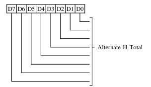
This register is used in low resolution (320-pixel) CGA modes and Hercules graphics modes.
