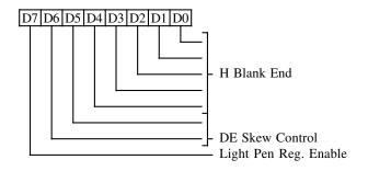
This register is used for all VGA and EGA modes. It is also used for 640 column CGA modes and MDA/Hercules text mode. In all 320 column CGA modes and Hercules graphics mode, the alternate register is used.
