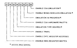
The Emulation Mode Register is located at offset 0FFh in the CRT Controller. This register can be accessed by first writing 0FFh in the CRTC Address Register (I/O address 3B4h/3D4h) and then accessing the CRTC Data Register (I/O address 3B5h/3D5h).
