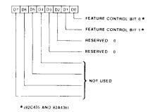
The Feature Control Register exists in both the 82C435 and the 82A436. This is normally a write only register in the 82A436. It can be read (in the 82C435) by setting the alternate read select bit in the 400 Line Register (CRF9 bit D7= 0) and then reading the CRTC Data Register at offset 0Eh. Feature Control Bits 0 and 1 from this register are also output on 82A436 output pins FCOUT0 and FCOUT1 respectively. These pins are typically used to drive the EGA Features Connecter.
