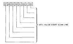
The Vertical Retrace Start Register is a 9-bit address which defines the scan line position of the VRTC pulse. The low order 8 bits are programmed through this register, while the high order ninth bit is programmed through the Overflow Register, CR7.
