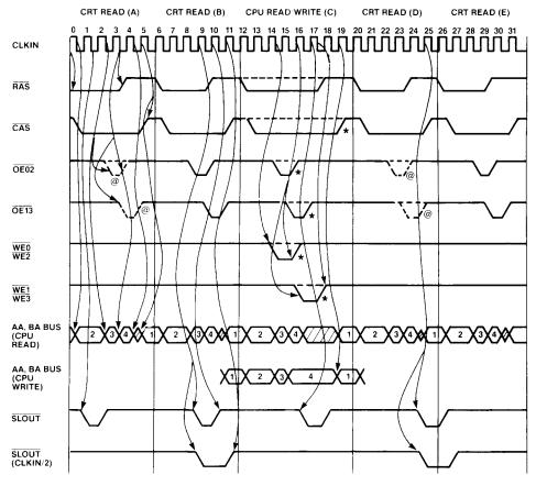
@ NOE<sub>x</sub> ACTIVE DURING CRT READ CYCLE A AND D ONLY FOR HIGH CRT BANDWIDTH MODE (SR0-D1:0) \* ONLY ACTIVE FOR VALID CPU/MEMORY READ/WRITE CYCLES
