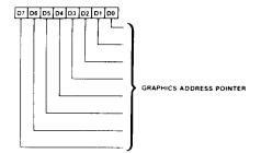
The Graphics Address Register is used to point to other registers in the Graphics Controller. The four least significant bits determine the register which will be pointed to in the next register write operation. When this register is read, D5, D6 and D7 are always '1'. D4 is '1' if D5, D6 and D7 were written as 1. D4 is '0' if D5, D6 or D7 were written as '0'.
