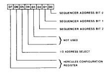
The Address Register is a three bit write-only register. When loaded with a binary value (pointer), it points to the data register where data is to be accessed.
