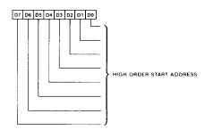
The Start Address is a 16-bit value which specifies the first word address in the display buffer for the screen refresh process. This display buffer address is mapped to the upper left corner of the screen. The Start Address High Register contains 8 high order bits of the address, while the Start Address Low Register specifies the other 8 low order bits. Byte resolution on this address can be achieved through the Extended Mode Register (CRF9 - bit D1).
