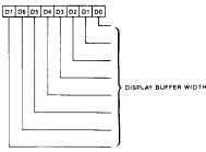
The Offset Register contents define the width of the Display Buffer currently used. This register is used to compute the memory starting address for the next display row (or scan line in graphics modes). The byte starting address of the next display row is computed as follows:
