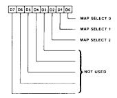
The contents of the Read Map Select Register represent the memory plane from which the CPU reads the data in read mode 0. This register does not effect the read operation performed through the Color Compare Register (read mode 1). The four memory maps are selected as follows:
