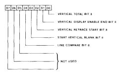
The CRT Controller Overflow Register contains the ninth bit (D8) of Vertical Total, Vertical Retrace Start, Start Vertical Blanking and Line Compare Registers.
