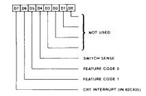
The EGA Input Status Register 0 exists in both the 82C435 and the 82A436. This register is located at I/O address 3C2h. In the 82A436, this is a read-only register and only bits 4, 5, and 7 are implemented. When this register is read in the EGA mode, the 82C435 drives the local data bus bit 7 and the 82A436 drives the other bits. In the CGA and Hercules modes, this register returns undefined values when read.
