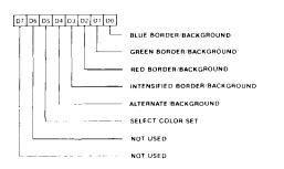
This registers serves as the CGA hardware palette register. This register is effective only when emulation is in progress (CRFF bit D2 = 1). This register can be disabled through the Emulation Mode Register (CRFF bit D3 = 0).
