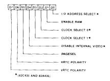
The EGA Miscellaneous Output Register is normally a write only register. It can be read by setting the alternate read select bit in the 400 Line Register (CRF9 bit D7 = 0) and then reading CRTC Data Register at offset 0Fh. The I/O Address Select bit (D0) can also be read at bit D5 of the Sequencer Address Register (I/O address 3C4h). This register performs the following functions:
