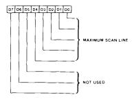
The contents of the Maximum Scan Line Register specifies the number of scan lines per character row. This actual number of scan lines per row is the contents of this register plus one.
