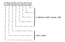
The Cursor Start Register defines the scan line within a character row where the cursor block is to begin. The first scan line for the cursor is the contents of this register.
