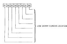
In conjunction with the Cursor Location High Register, the Cursor Location Low Register defines the low order 8 bits of the cursor location.
