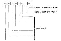
The Hercules Configuration Register is effective only when Hercules emulation is in progress (CRFF bit D2 = 1) and EGA Misc Output Register bit D0 = 0. Bits D0 and D1 are read at bits D6 and D7 respectively in the Sequencer Address Register (I/O Address 3C4h).
