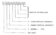
The Vertical Retrace End Register performs multiple functions, as described below:
