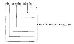
The Cursor Location address is a 16-bit value. The 8 high order bits are programmed in the Cursor Location High Register. The other 8
