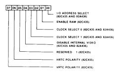
The EGA Miscellaneous Register exists in both the 82C435 and the 82A436. This register is located at I/O address 3C2h. In the 82A436, this is a write only register and only bits 0, 2, 3, and 4 are implemented. These bits are also present in the 82C435. When this register is read, the 82C435 drives the local data bus and the 82A436 transfers the contents of the local data bus to the CPU.
