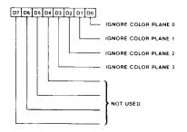
Any bit in the Color Don't Care Register that is set to 0 indicates that the corresponding bit in the Color Compare Register is a don't care in read mode 1. Any bit set to 1 enables the corresponding bit in the Color Compare Register.
