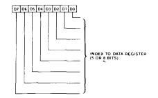
The CRT Controller Registers are all located at two byte addresses in the CPU I/O space. The registers are accessed by first writing a pointer to the actual data register into the CRT Controller Address Register and then accessing the CRT Controller Data Register. The Address Register is located at I/O address 3B4h/3D4h. The data registers are all located at I/O address 3B5h/3D5h. The exact address 3Bx/3Dx is selected thorough bit D0 of the EGA Misc. Output Register.
