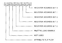
D0-D4 are used to point to the internal data registers in the Attributes Controller.
