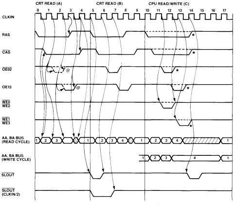
@ NOEx ACTIVE DURING CRT READ CYCLE A ONLY FOR HIGH CRT BANDWIDTH MODE (SR0-D1=0) \*ONLY ACTIVE FOR VALID CPU/MEMORY READ/WRITE CYCLES
