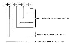
The contents of the End Horizontal Retrace Register define the character count at which the Horizontal Retrace Pulse becomes inactive.
