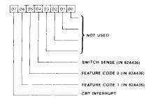
Parts of the Input Status Register 0 exist in both the 82C435 and the 82A436. The data path to the CPU from the 82C435 always goes through the 82A436. When the CPU reads this register, the 82A436 reformats the status data put out by the 82C435 and passes the final status to the CPU.
