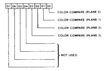
If the Graphics Mode Register is set to Read Mode 1, each bit of data read from the display memory planes 0-3 is compared to bits D0 through D3 programmed in the Color Compare Register and the Color Don't Care Register. A match between the memory data and the Color Compare Register (for the bits as specified in the Color Don't Care Register) results in a logical 1 being output on the corresponding data bus bit. Following is an example to illustrate the mechanism:
