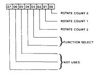
The Data Rotate Register is used to perform a rotate function on the data written by the CPU. If the Graphics Mode Register is programmed for write mode 0, then the value in the Rotate Count Field represents the number of bits the CPU data will be rotated (right) during the CPU write cycles. The CPU data bits are first rotated and then subject to the logical operation as specified in the Function Select Field.
