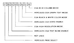
All the bits in the Hercules/CGA Mode Control Register are effective only when emulation is in progress (CRFF bit D2 = 1). When CGA emulation is in progress (EGA Misc. Output Register bit D0 = 1), then this register functions as the CGA Mode Register and is located at I/O address 3D8h. When Hercules emulation is in progress (EGA Misc. Output Register bit D0 = 0), then this register functions as the Hercules Mode Register and is located at I/O address 3B8h.
