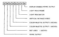
The Input Status Register I exists in both the 82C435 and the 82A436. This register changes address and format in the EGA, CGA and Hercules modes. In EGA mode this register is located at I/O address 3BAh/3DAh. In CGA mode this register is located at I/O address 3DAh. In Hercules mode this register is located at I/O address 3BAh. When this register is read, the 82C435 and 82A436 drive different bits in the three modes as follows:
