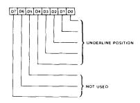
The Underline Location Register specifies the scan line within a character row at which the underline will appear for underlined characters. The value in the register should be one less than the desired scan line number.
