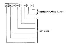
The Graphics A Position Register selects the CPU data bus signals and directs them to/from display memory planes 0 and 1. This register should normally be programmed to 00h to select D0 and D1 for display memory planes 0 and 1 respectively.
