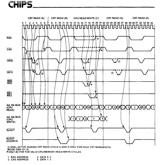
Figure 7. Memory Cycle Division for Low CRT Bandwidth Mode (SR1-D5=0), 9 Dots/Character
