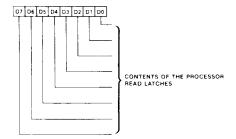
There are four byte-wide latches inside the 82C435. These latches are set whenever the CPU reads the display memory. The contents of these latches are subsequently used for the logical operations in the CPU write cycles. In order to completely determine the context of the 82C435, these latches can be read by the CPU as four byte-wide registers in the Graphics Controller address space. The registers at offset F8h-FBh reflect the contents of
