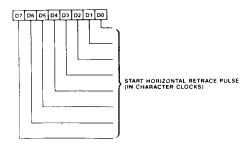
The Start Horizontal Retrace Pulse Register defines the character position at which the Horizontal Retrace Pulse becomes active. It is used to center the monitor screen horizontally. The value in the register is the character count at which the Horizontal Retrace Pulse becomes active.
