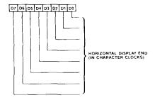
The Horizontal Display Enable End Register defines the number of characters to be displayed per horizontal line. The actual characters displayed per horizontal line is one more than the contents of this register.
