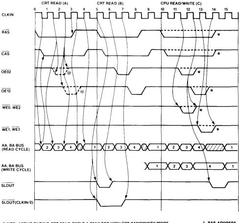
@ NOE, ACTIVE DURING CRT READ CYCLE A ONLY FOR HIGH CRT BANDWIDTH MODE (SR0-D1=0)  $\star$  ONLY FOR CPU-MEMORY RD/WR CYCLES 1. RAS ADDRESS 2. CAS ADDRESS 3. DATA 0, 2 4. DATA 1, 3
