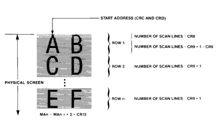
CR8 = PRESET ROW SCAN CR9 = MAXIMUM NUMBER OF SCAN LINES/CHARACTER ROW CRC, CRD = DISPLAY BUFFER START ADDRESS CR13 = DISPLAY BUFFER WIDTH (OFFSET) MA<sub>n</sub> = MEMORY ADDRESS FOR FIRST CHARACTER IN THE nth ROW
