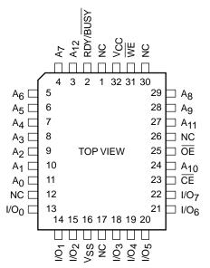
**TSOP Top View (8mm x 13.4mm) (T13, H13)**
