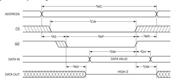
Figure 3. Early Write Cycle Timing
