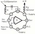
NOTE: Pin 4 connected to case.
