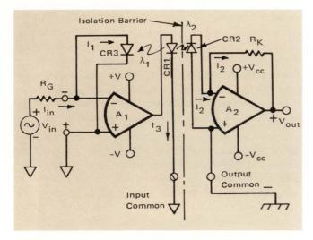
FIGURE 3. Improved Linear Isolator.
