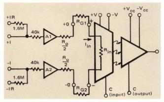
FIGURE 5. Simple Model of 3652.
