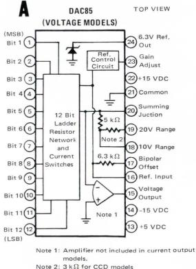
Note 2: 3 k $\Omega$  for CCD models 5 k $\Omega$  for CBI models
