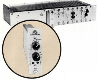
The 3640 offers excellent performance at a surprisingly low cost. The direct-coupled, differential input stage provides resolution of microvolt signals through the use of a low noise, monolithic amplifier. Low DC input drift is assured by proprietary input stage balancing techniques. Linearity of 0.01% and gain accuracy of 0.1% are achieved through the use of heavy negative feedback and precision, high stability resistors.
