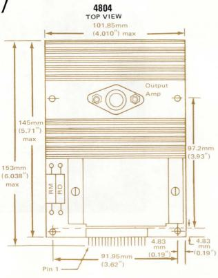
Material: Extruded, black-anodized, aluminum heat sink and discrete components mounted on glass epoxy printed circuit board.
