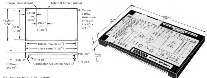
MATING CONNECTOR: 7200MC CASE MATERIAL: INSULATED STEEL CONNECTOR PINS: GOLD FLASHED WEIGHT: 200 GRAMS (7 OZ.)
