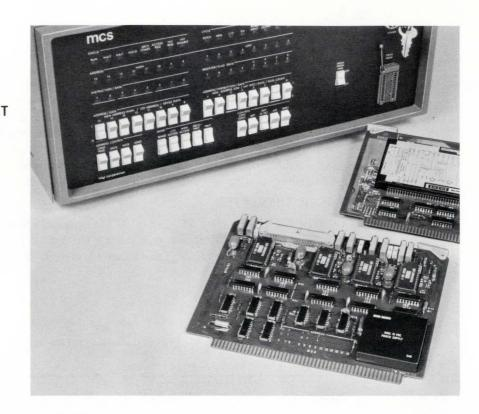
and SDM851 modular data acquisition systems are used to implement these systems. The data acquisition systems include an input multiplexer, instrumentation amplifier, sample/hold and 12 bit A/D converter along with all the necessary timing, decoding and control logic. The model 546 DC/DC converter (+5V to  $\pm 15V$ ) is also used so that only the Intellec's +5VDC power supply is required.
