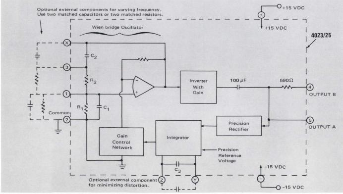
SIMPLIFIED SCHEMATIC DIAGRAM OF MODEL 4023/25
