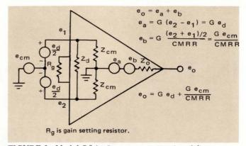
FIGURE 2. Model Of An Instrumentation Amplifier.
