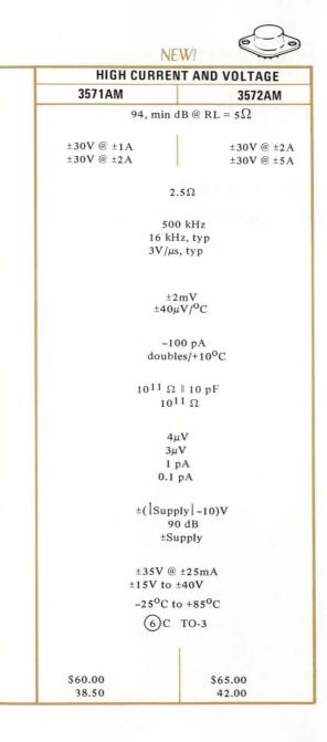
Specifications typical at 25<sup>0</sup> and rated supply voltage unless otherwise noted.
