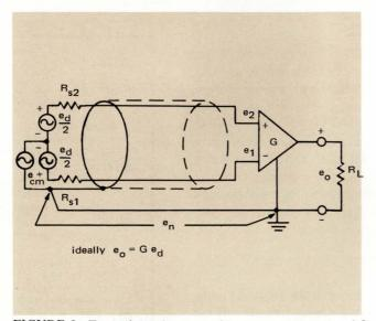
FIGURE 3. Typical Application of Instrumentation Amplifier.
