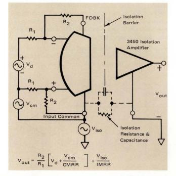
FIGURE 1. Typical Isolation Amplifier Application.
