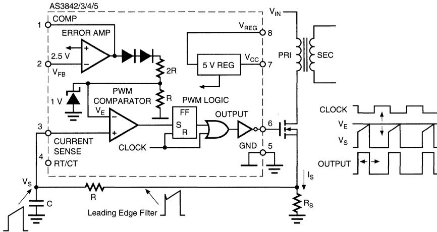
Figure 20. Current Sense/PWN Latch Circuit and Waveforms
