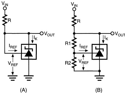
**Figure 2.** AS431 Precision Voltage Reference
