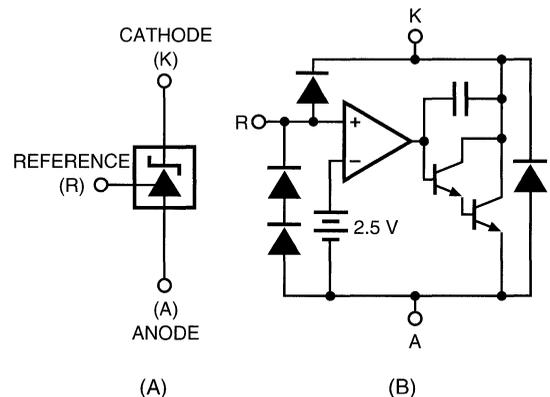
Figure 1. AS431 A) Schematic Symbol
