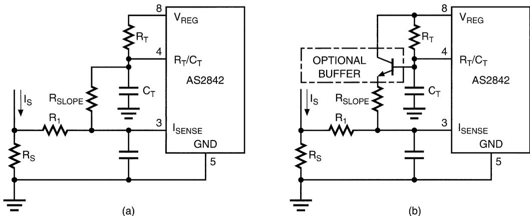
Figure 23. Slope Compensation
