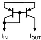
**Figure 2.** Simple PNP Current Source. Has Slower Frequency Response, and up to ±15% Tolerance Error.
