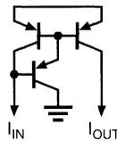
**Figure 3.** Widlar Current Source, Moderate Frequency Response.
