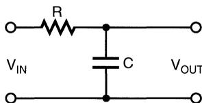
$$T(S) = \frac{V_{OUT}(S)}{V_{IN}(S)} = \frac{1}{RCs + 1}$$
