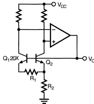
Figure 11. Brokaw Band Gap Reference.
