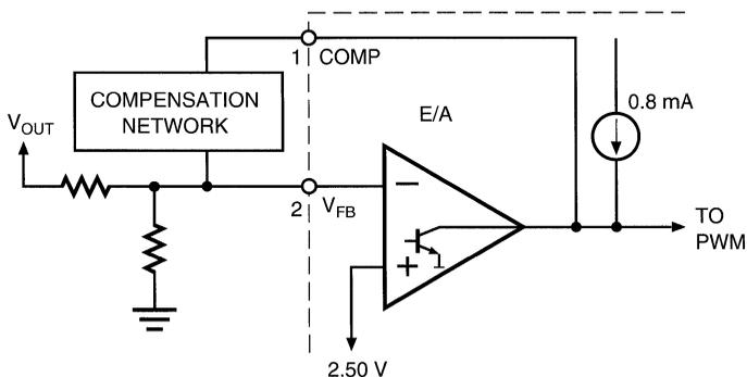
Figure 17. Error Amplifier Compensation
