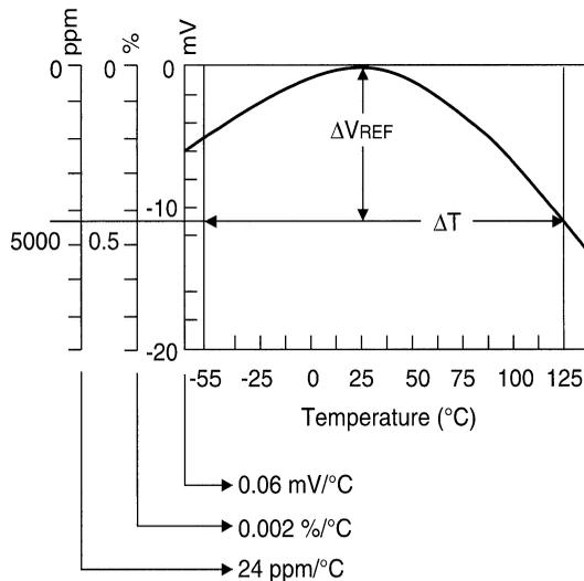
$$\bullet \text{ TC in mV}/^\circ\text{C} = \frac{\Delta V_{REF} \text{ (mV)}}{\Delta T_A}$$
