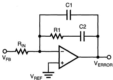
$$G3(s) = \frac{V_{ERROR}}{V_{FB}} = \frac{1 + R1C2}{R_{IN}(C2 + C1) + SR1(C2 \bullet C1)}$$
