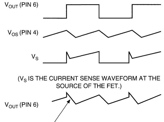
THIS IS THE RESULT OF SUPERIMPOSING V<sub>OS</sub> ON V<sub>S</sub>. THIS LEADING EDGE VOLTAGE SPIKE COULD FALSELY TRIGGER THE CURRENT SENSE COMPARATOR AND CAUSE NOISE PROBLEM.
