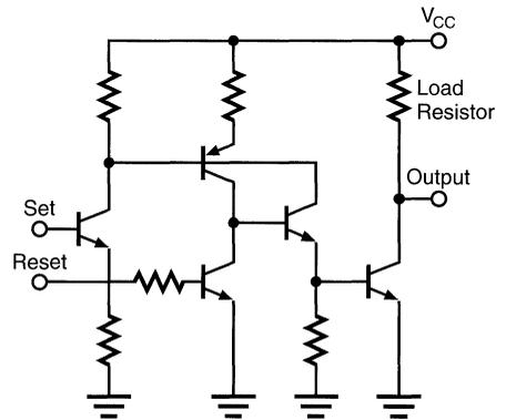
Figure 18. Four Layer Latch Flip-Flop
