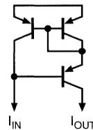
**Figure 4.** Wilson Current Source, Fast Frequency Response.
