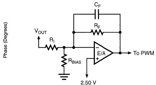
Figure 19. A Typical Compensation Network
