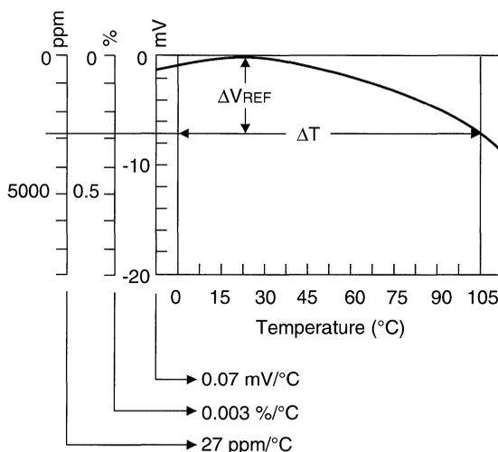
$$\bullet \text{ TC in mV}/^\circ\text{C} = \frac{\Delta V_{REF} \text{ (mV)}}{\Delta T_A}$$
