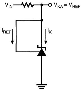
Figure 1a. Test Circuit 1
