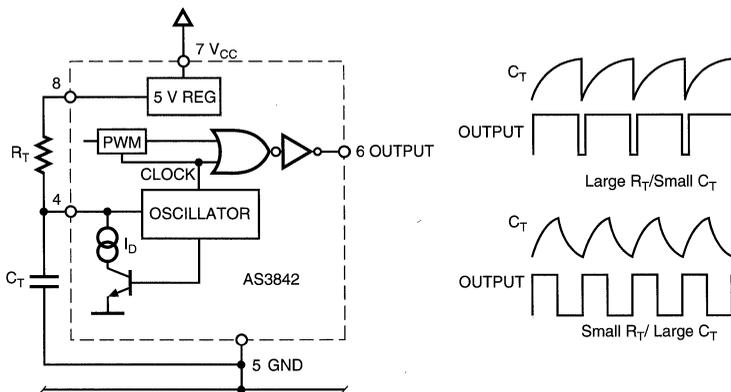
Figure 15. Oscillator Set-up and Waveforms
