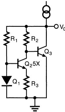
Figure 10. Widlar Band Gap Reference.
