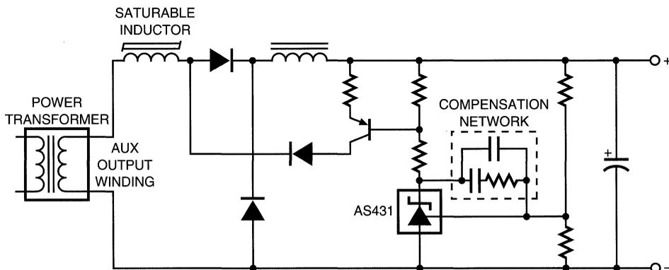
Figure 5. An AS431 Controlled MagAmp Post Regulator
