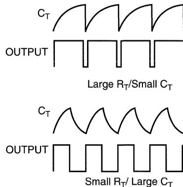
Figure 15. Oscillator Set-up and Waveforms
