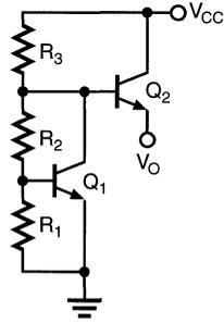
Figure 9.  $V_{BE}$  Multiplied Regulator.
