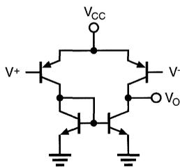
**Figure 6.** Simple NPN Type Comparator Input Stage.
