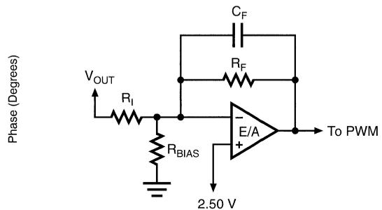
Figure 19. A Typical Compensation Network
