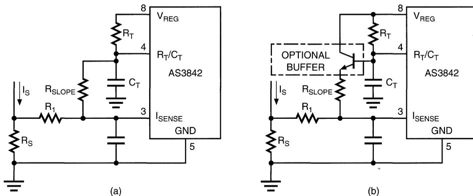
Figure 23. Slope Compensation
