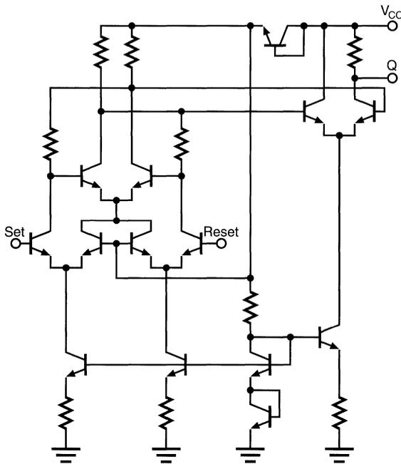
Figure 17. Fast, ECL Flip-Flop
