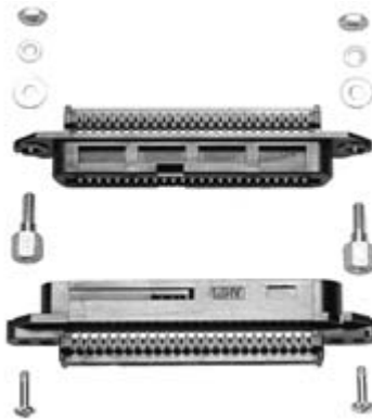
Screw Lock Hardware Kit Part Number 552568-1 (For rear panel mount applications, max. panel thickness shall be .062 [1.57].) (One kit required per assembly)
