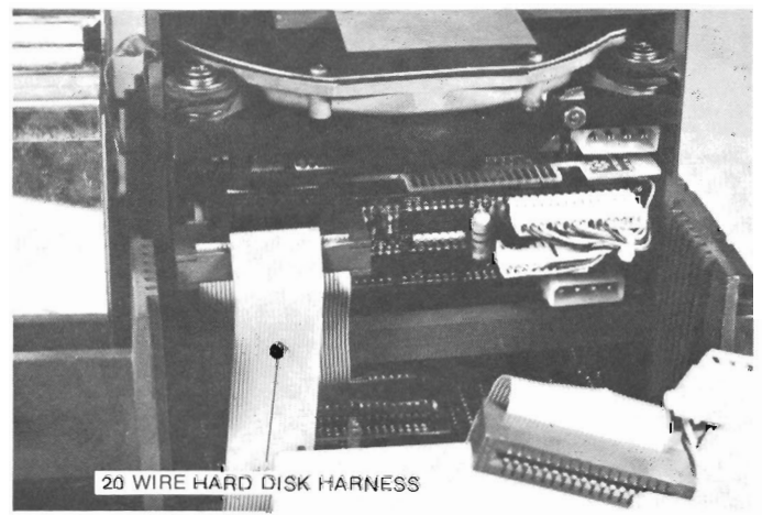
PHOTO 5.G (a) - Attach 20-wire hard disk cable.
